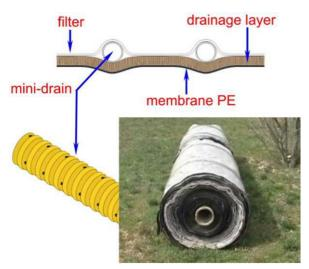
Figure 2. Geocomposite Draintube FT/PE structure
