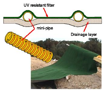
Figure 6. Geocomposite DRAINTUBE 700PP FT 1 D16 UV 2 GREEN
