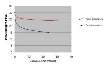
Figure 7. Loss tensile strength of the geocomposite installed in Villeparisis versus exposure time
