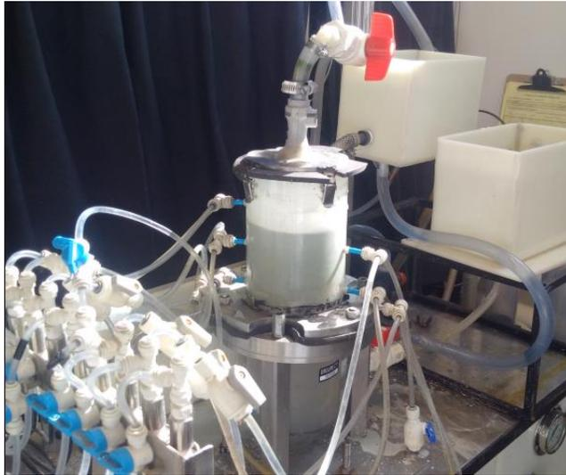
Figure 7 Set-up of the filtration test (Gradient Ratio, ASTM D5101)
