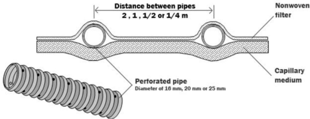
Figure 1 Multi-Linear drainage geocomposite
