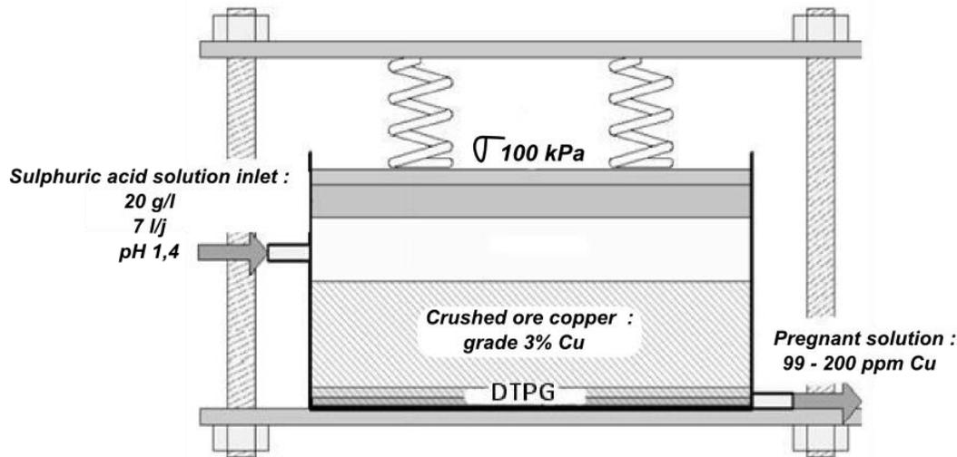
Figure 2 Cross-section of an experimental leaching cell. During 90 days, acid leachate percolates through the ore then the MLDG
