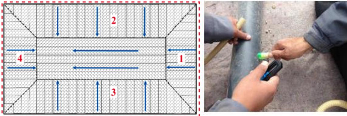
Figure 12: orientation of the MLDG and connection using connectors (photo courtesy AfiteX-Texel)
