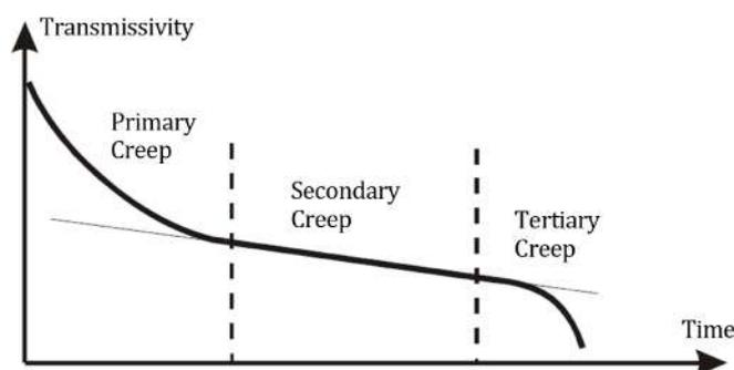
FIG 3 – Creep behaviour of planar drainage geosynthetics (Saunier and Blond, 2010).
