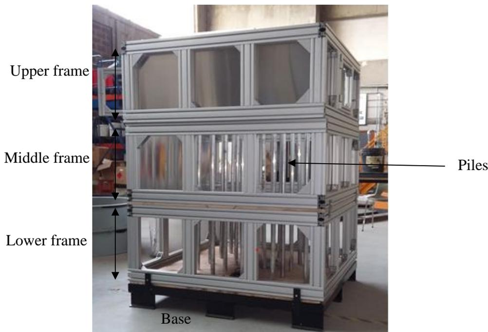
Figure 1. Small-scale device
