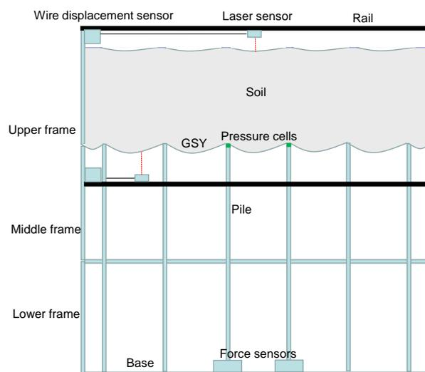
Figure 3. Monitoring for the test without soft soil
