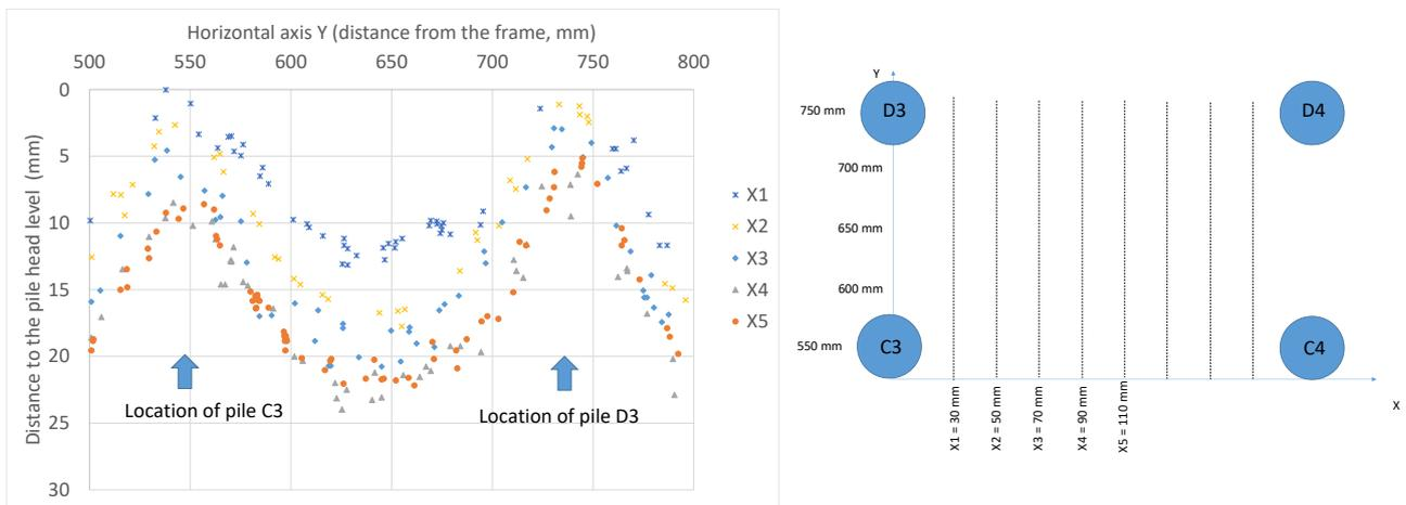
Figure 6. Deflection of the geosynthetic in the central grid under a layer of 20 cm of sand
