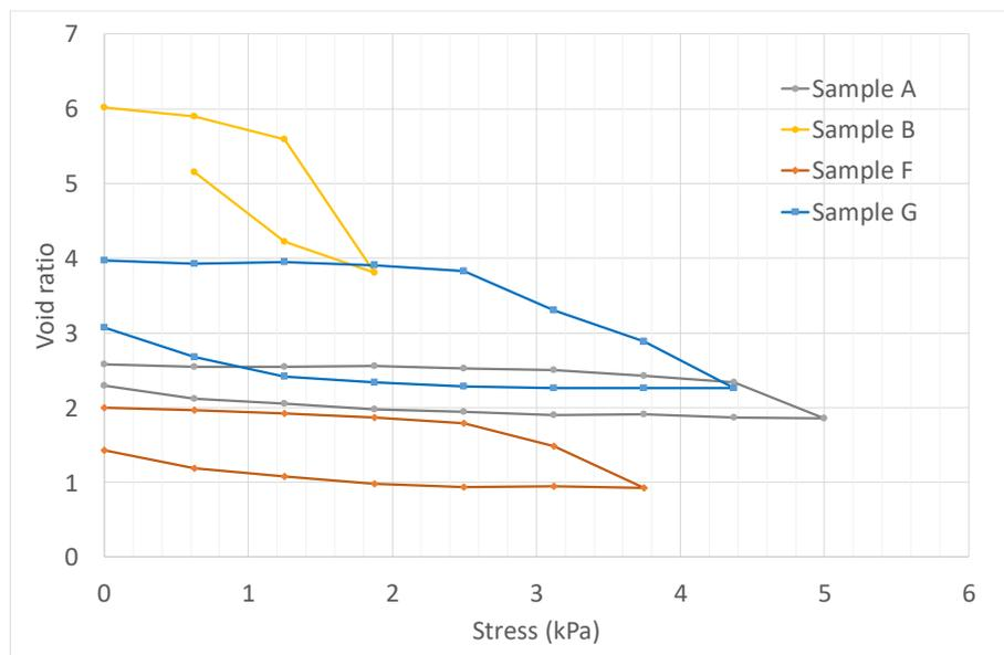
Figure 5. Compressibility tests
