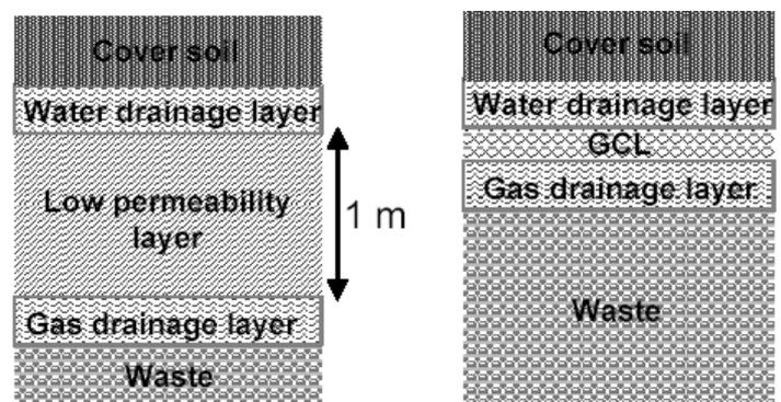
Figure 1. Typical semi-permeable landfill cover with low permeability layer or GCL.
