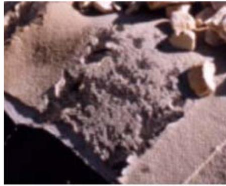
Figure 5. Damage to the geotextile filter caused by UV rays
