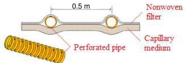
Figure 1. Daintube drainage geocomposite
