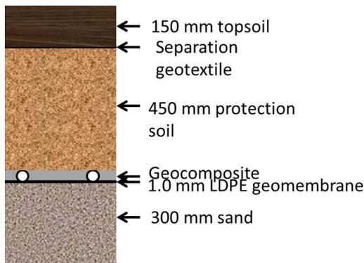
Figure 2. Cross section of landfill cover
