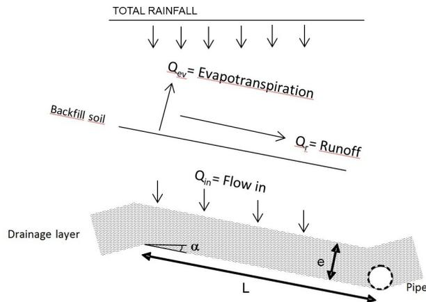
Figure 9. Schematic drawing of the hydraulic function of the drainage layer (ADEME 2001).
