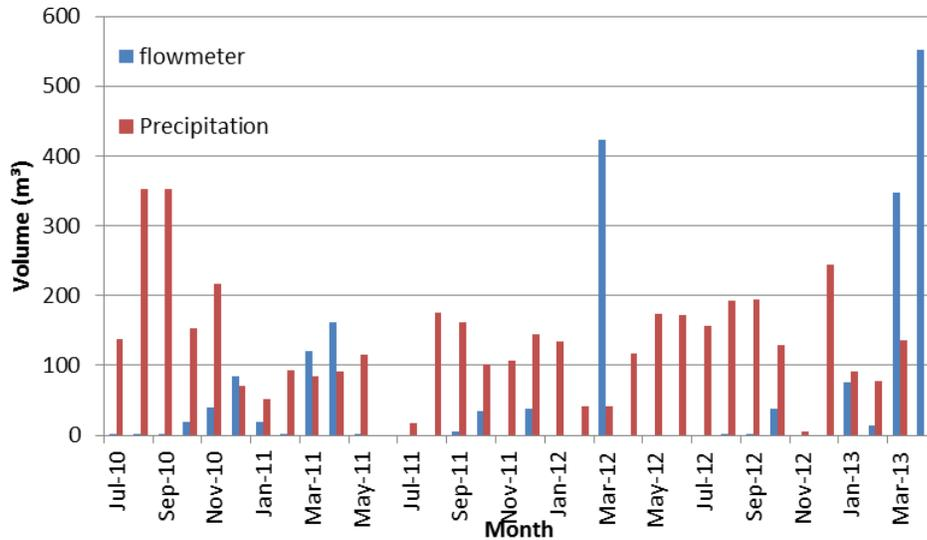
Figure 5. Volume of monthly flow through flowmeter, and calculated volume of rainfall over the area of the test pad.
