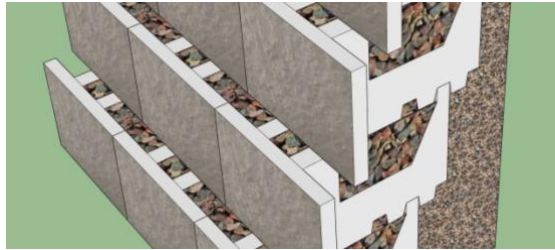
Figure 6. Ballast fill material.
