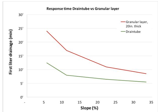
Figure 6: Drainage response time Draitube vs granular layer
