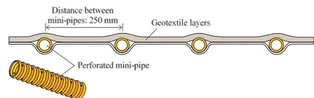
Figure 1. DRAINTUBE geocomposite description
