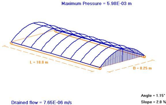
Figure 9: Daintube Flow capacity
