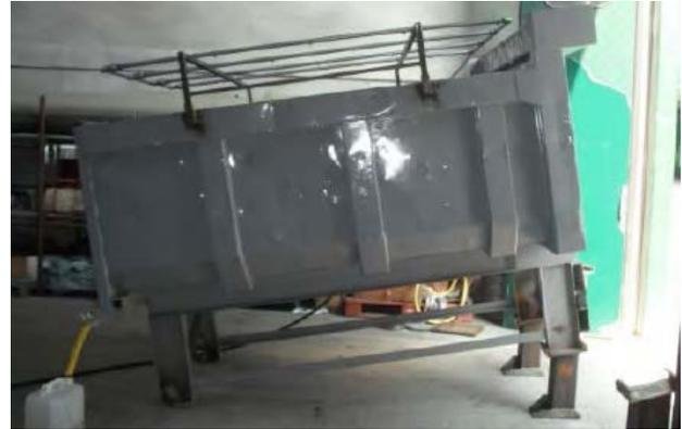
Figure 5: inclinable open box with rainfall simulator
