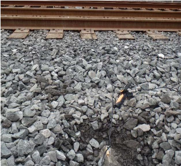
Figure 10: Video inspection using a video endoscope
